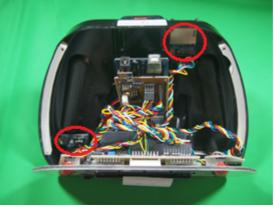
Remove all the cables from the mother board. You can remove the old SD card reader and earphone mount (red circles). n
