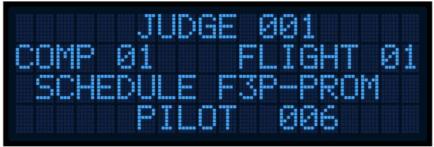
You can skip from one item to another with the rotary knob and then change the values with "-" or "+" button. Once you are happy with the values, press "Valid" until you are on the pilot number (pilot number is blinking). The Notaumatic proceeds to some checkings and will alert you in case of an issue. If everything is OK, you are now ready to enter scores. (See previous screen)
