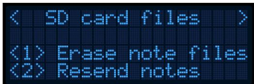
The device stores the scores for each manoeuvre for each flight. Before starting a new contest, the existing stored scores must be deleted.
