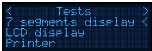
A list of available tests is displayed by pressing up and down on the joystick. Press the left joystick to select a test. A long press on the center of the joystick will exit the results of a test.
