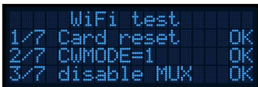
Displays the different phases in a drop-down list. The WiFi card integrated into the Notautomatic unit connects to the access-point as described on the SD card, and then tries to connect to the specified server.
