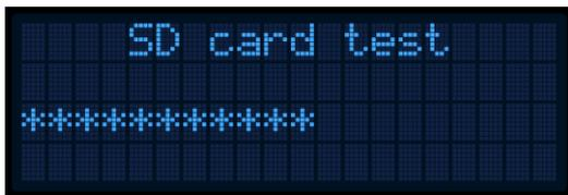
Reads all files on the SD card. The number of files read is displayed at the end of the test. In a second step, the physical characteristics of the SD card are displayed.
