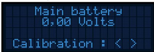
Displays the main battery voltage. The accuracy of this measurement depends on the internal components and a calibration value. This calibration factor can be adjusted with the joystick left and right.
