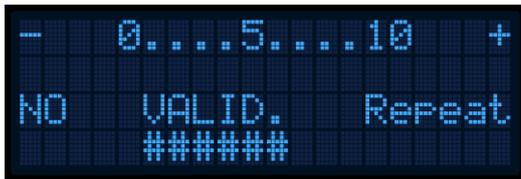
The display shows the result of pressing buttons on the Notautomatic unit. In this example the <Valid> key has been pressed.
