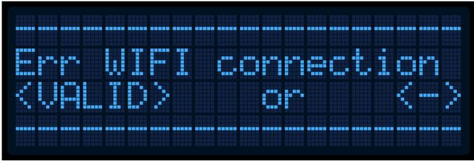
If there is a problem, an error message will be displayed. Refer to the "List of errors" at the end of this manual. You can return to the setup screen with the <-> key.
